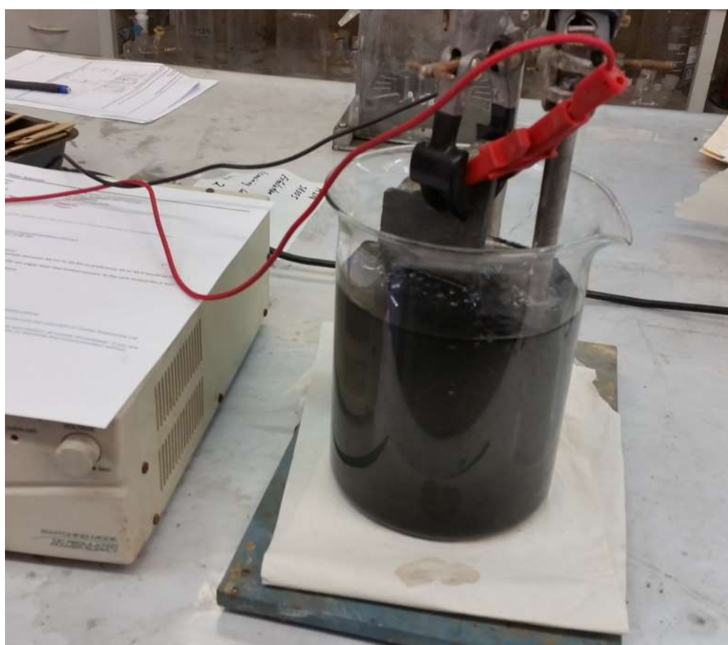
Figure 3: Exfoliation of HD002 Core
