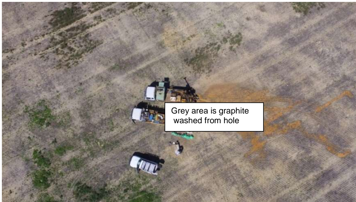
Figure 9: Picture showing aircore drilling and water flow
