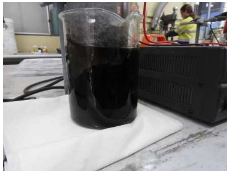
Figure 2: Exfoliation of core from HD018.
