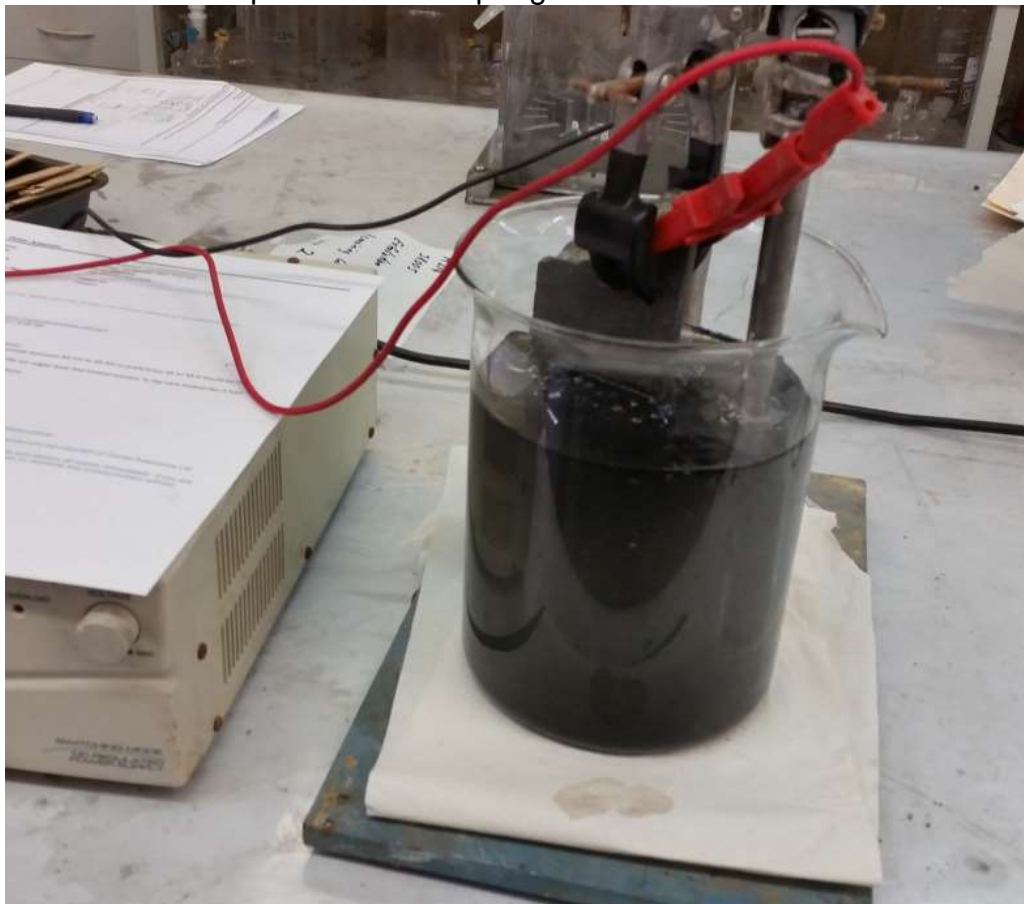
Figure 6: Exfoliation of HD002 Core
