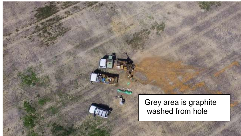
Figure 2: Picture showing aircore drilling and water flow
